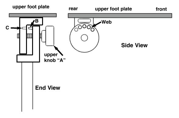
To adjust the angle of the upper plate of the footstand, release the upper knob "**A**" until the tapered pin "**B**" is completely out of recess "**C**".
