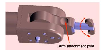
2. Insert the arm assembly into the attachment joint until the telescoping rod will allow for the required manipulator movement.
