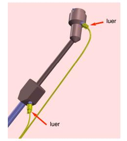
3. Connect the branched line to the two luers of the arm assembly.
