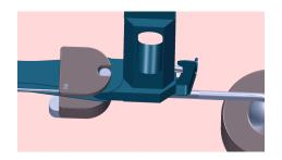
6. Tighten the joining screw.
